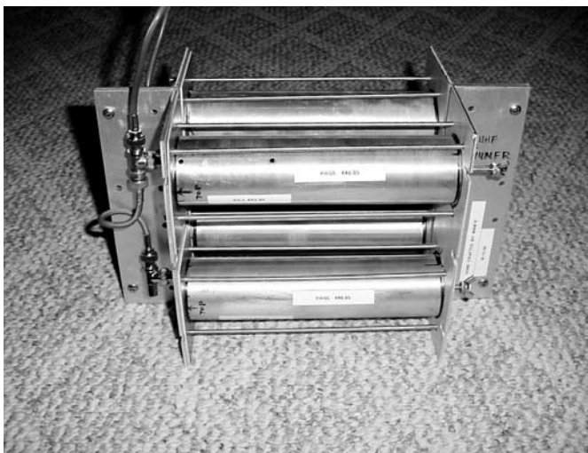
Photo I — This side view of the completed duplexer assembly shows all four duplexer cavities.
