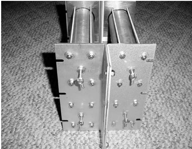
Photo G — This end view of the completed pair of cavities shows the bandpass tuning adjustment all thread rods through the angle brackets.
