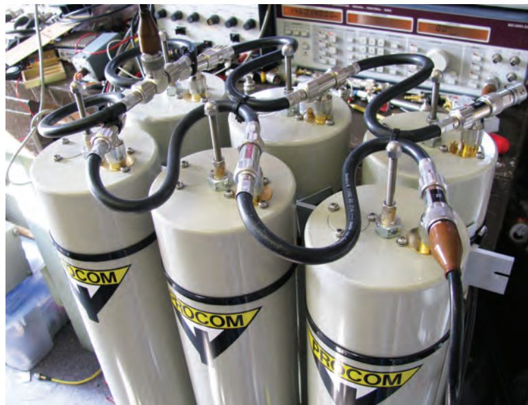
PHOTO 1: DPF2/33 2m band 6 cavity duplexer.
