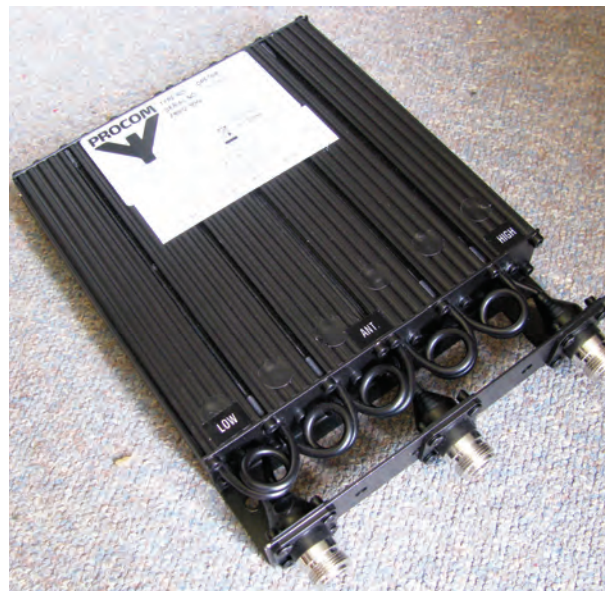
PHOTO 2: DPF70/6 70cm band 6 cavity duplexer.
